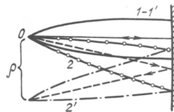
FIG. 5. The Interpretation of the intensification of intensity fluctuations and of the shift in the temporal spectrum accompanying reflection from a mirror surface.
