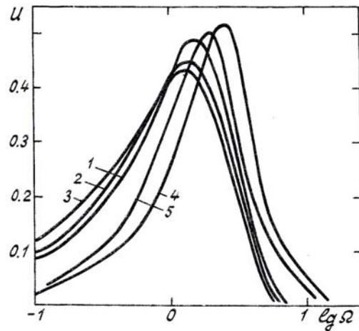
FIG. 3. The normalized spectrum of intensity fluctuations  $U = fW(f, \tilde{\rho}) / \sigma_{\perp}^2$ .
