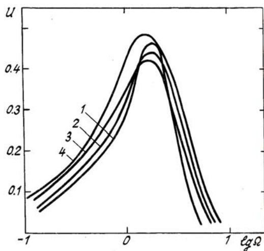
FIG. 4. The normalized spectrum of intensity fluctuations  $U = fW(f, \bar{\rho}), \sigma_1^2$ ,  $v_{\perp} = 3.4-3.9$  m/sec.  $\sigma_v = 0.4-0.7$ .  $\sigma_v = 0.4-0.7$ , For  $\beta_0 > 1$   $\bar{\rho} = 0.1$  (1),  $\bar{\rho} = 0.6$  (2), and  $\bar{\rho} = 0.9$  (3); for  $\beta_0 < 1$   $\bar{\rho} = 0.1$  (4).
