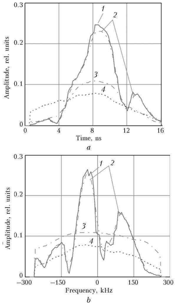
**Fig. 4.** Cross sections of the envelope of normalized MRF of the model (curve 1) and of the normalized estimates of MRF formed while using PCM-signal (2), chirp-signal (3), and simple signal (4).
