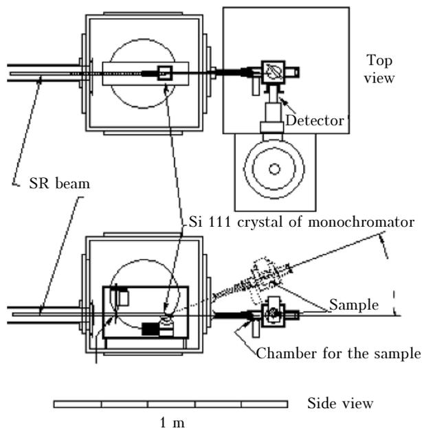
Fig. 5. Block-diagram of the setup for scanning roentgen-fluorescent analysis of annual rings of coniferous trees.
