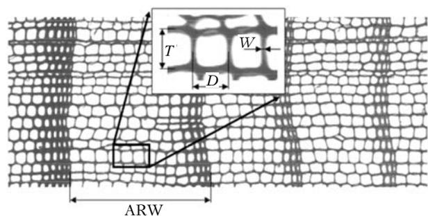
Fig. 4. Section of pine sample: ARW is the annual ring width;  $D$  and  $T$  are the radial and tangent cell sizes;  $W$  is the thickness of the doubled cell wall.
