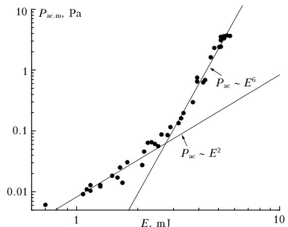
**Fig. 3.** Peak acoustic pressure as a function of the laser pulse energy.
