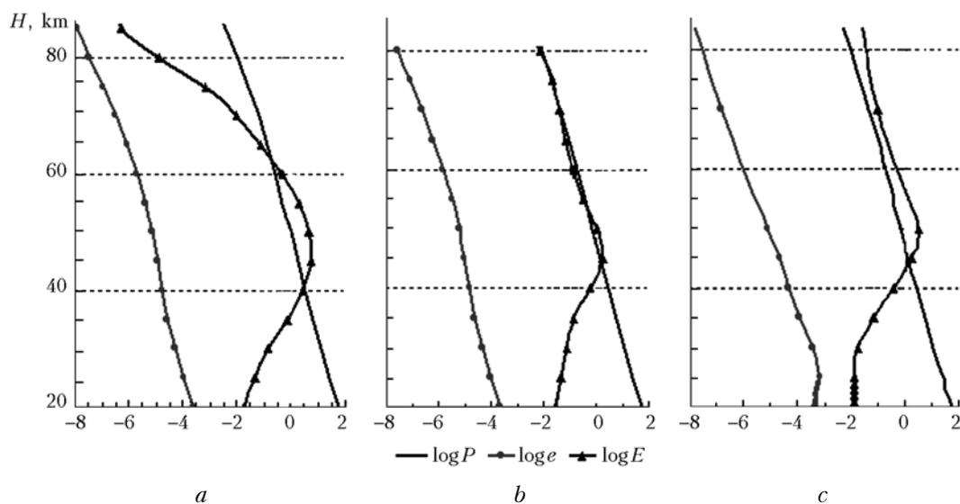
**Fig. 3.** Water content  $e$  (mbar), the pressure of saturated water vapor above ice  $E$ , and atmospheric pressure  $P$  at an altitude of 20–80 km.
