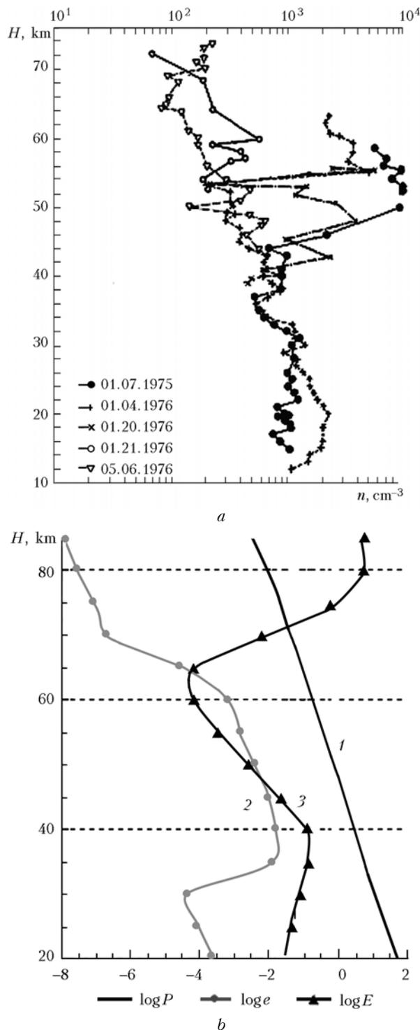
Fig. 8. Content of positive ions (a) and water (b) in stratopause for the days of anomalous absorption in ionosphere:  $\log P$  (1);  $\log e$  (2);  $\log E$  (3).
