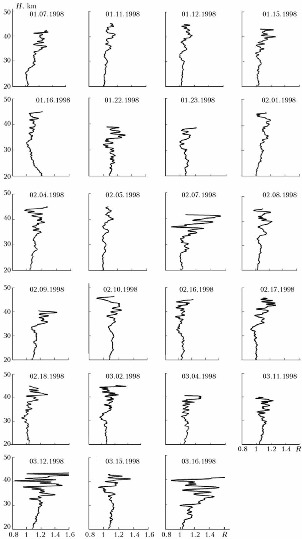
Fig. 1. Profiles of aerosol scattering ratio  $R$ , obtained at the Tomsk lidar station for January–March, 1998 [Ref. 2].
