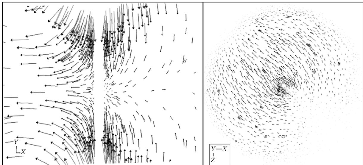
**Fig. 3.** The field of the gas motion velocity, caused by thermal slip on nonhomogeneously heated thread holders and on the thread itself. To the left, the velocity field plane passes through the holders (they are inside the visual zone); to the right, the velocity field plane is perpendicular to the thread at its middle point.
