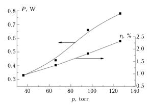
Fig. 2. The dependence of excilamp radiation average power and efficiency in  $Xe-Br_2 = 400-1$  gas mix on the pressure of inertial gas.
