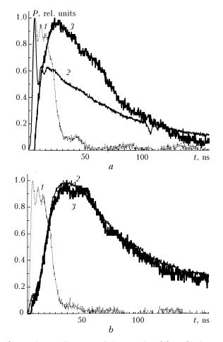
**Fig. 1.** The oscillograms of laser pulse (1) and plasma luminosity pulses on the surface of heavy (a) and liquid (b) Wood alloy at 200–600 (2) and 340–600 nm (3) wavelengths in the neon atmosphere at a pressure of 370 Torr.
