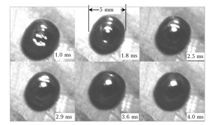
Fig. 2. Dynamics of relaxation of the liquid gallium drop surface. Exposure time of each frame is 1  $\mu$ s, the interframe times are: 1; 1.8; 2.5; 2.9; 3.6; and 4 ms after the irradiation. The beam incidence is normal to the picture. The ablation region is in the drop center.
