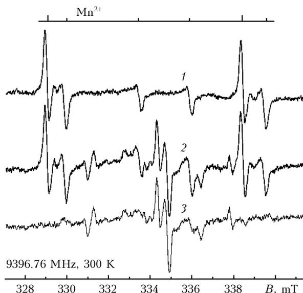
**Fig. 3.** EPR spectrum of organic radicals on the  $\text{CaCO}_3$  surface: standard sample (1); exhibited sample (2); a focused signal of organic radicals in the exhibited sample (3).  $B$ , mT (polarizing magnetic field in millitesla).
