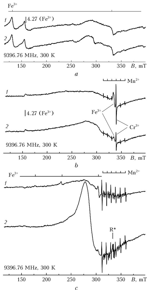
**Fig. 2.** EPR spectra of standard (1) and exhibited (2) samples for sorbents:  $\text{Al}_2\text{O}_3$  (a),  $\text{MgO}$  (b),  $\text{CaCO}_3$  (c).  $B$ , mT (polarizing magnetic field in millitesla).
