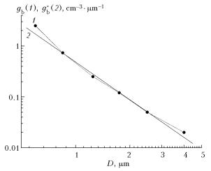
**Fig. 4.** Particle size distribution function for the background component of arid aerosol in size range  $0.5-5.0 \ \mu\text{m}$  (1) according to the data of measurements on August 14, 2007 in Kharabali, Astrakhan Region (the natural reserve "Berli Peski") and the approximating power distribution (2) with an index of -2.5.
