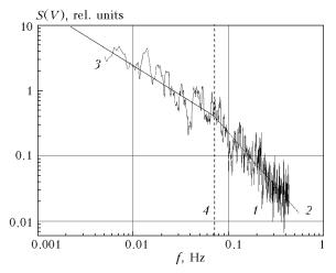
**Fig. 6.** Spectral power density of wind velocity module (1) by measurements on August 14, 2007: the boundary of turbulence regimes (4); approximating power spectra (2), (3).
