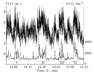
Fig. 1. Fluctuations of the horizontal wind velocity modulus (1) and number concentration of aerosol particles, whose sizes are more than 0.5  $\mu$ m (2) according to the measurements on August 14, 2007 in the natural reserve "Berli Peski," Astrakhan Region (I, II, III, and IV are distinguished gusts and aerosol spikes).
