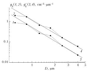
Fig. 5. Particle size distribution function for the arid aerosol component, generated on the underlying surface in size range of  $0.5-5.0 \ \mu\text{m}$  (according to the measurement data on August 14, 2007 in Kharabali district, Astrakhan Region): average by four spikes (1) and average by four maximal spikes (2). Approximating power spectra have indices of -2.25 (3) and -2.17 (4).
