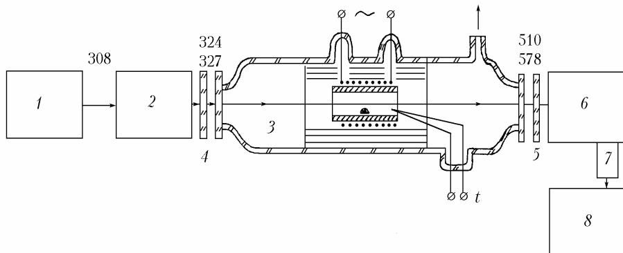
**Fig. 1.** Block diagram of the experiment: excimer laser 1, dye laser with frequency doubling 2, cell 3, UV filter 4, visible filters 5, monochromator 6, photodetector 7, and Brookdeal system for detection of signals 8.
