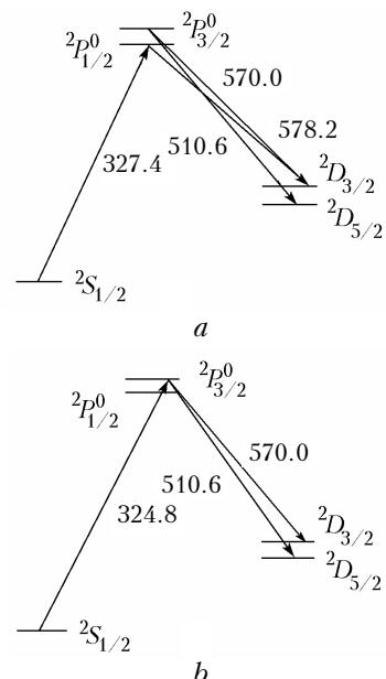
**Fig. 2.** Optical transitions in the Cu atom observed at optical excitation of the mixture of copper vapor and inert gases at  $\lambda = 327.4$  (a) and  $324.8$  nm (b).
