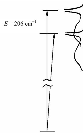
**Fig. 4.** Components of the copper resonance doublet and conditional form of their excitation function.
