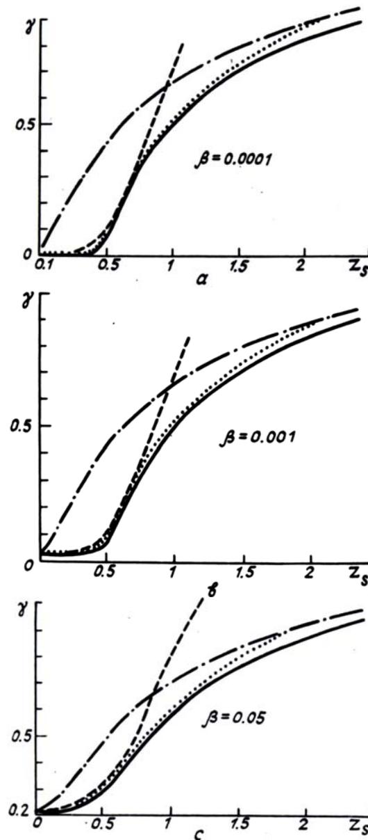
FIG. 2. The angular divergence  $\gamma$  versus the effective thickness of the nonlinear layer  $z_s$  for optimally focused (solid curve) and collimated (dot-dashed curve) beams as well as for a beam with predistortion  $\varphi_k$  (dashed curve) and a beam with phase correction determined by the programmed-phase-correction algorithm with a reference plane wave (dotted curve).
