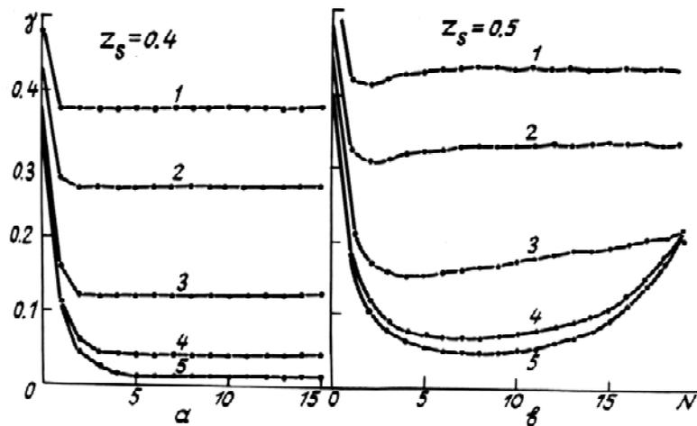
FIG. 1. The angular divergence  $\gamma$  versus the number of iterations  $N$  for several values of  $\beta$  ( $\beta = (L_R/L_D)^2$ ):  $\beta = 0.5$  (1), 0.05 (2), 0.01 (3), 0.001 (4), and 0.0001 (5);  $z_c = 0.4$  (a) and 0.5 (b).
