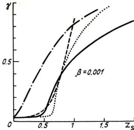
FIG. 3. The angular divergence  $\gamma$  as a function of  $z_s$  with nonlinearity of the wind type.  $f(z)$  is given by Eq. (6): collimated beam (dot-dashed curve), beam with predistortion  $\varphi_k$  (dashed curve), optimally focused beam (dotted curve);  $f(z)$  represented by Eq. (5): optimally focused beam (solid curve).
