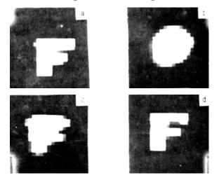
FIG. 1. Reconstruction results from 80 images: from unquantized images (a); from images quantized into 4, 8, and 16 levels, respectively, (b), (c), and (d).
