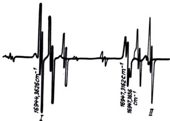
FIG. 2. Absorption spectra of \text{H}_2\text{O} vapor (1) (heavy lines) and a mixture of \text{H}_2\text{O} and \text{D}_2\text{O} vapor (1) (light lines) between 16\,948.002\text{ cm}^{-1} and 16\,943.128\text{ cm}^{-1} .
