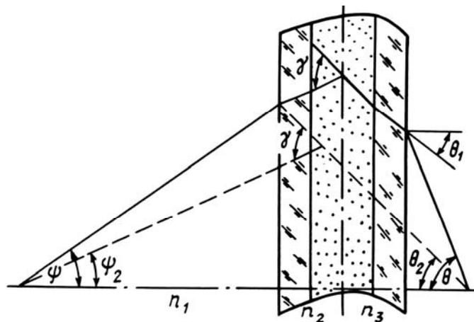
FIG. 1. Geometric diagram of measurements of the PSF in the method of angular scanning.  $\theta$  are the angles of emergence from a point object.
