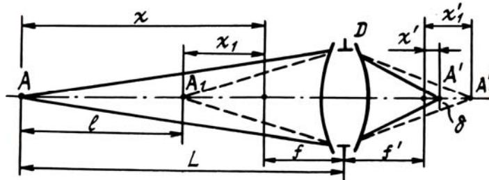
FIG. 3. The geometric scheme for calculating the scattering spot in the method of angular scanning.
