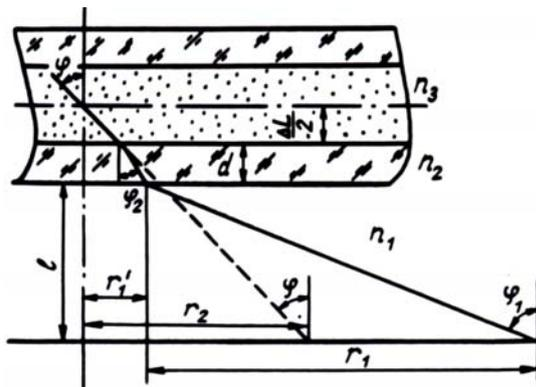
FIG. 2. The geometric diagram of measurements of the PSF in the method of spatial scanning.  $\varphi_1$  are the angles of emergence from a point test object.
