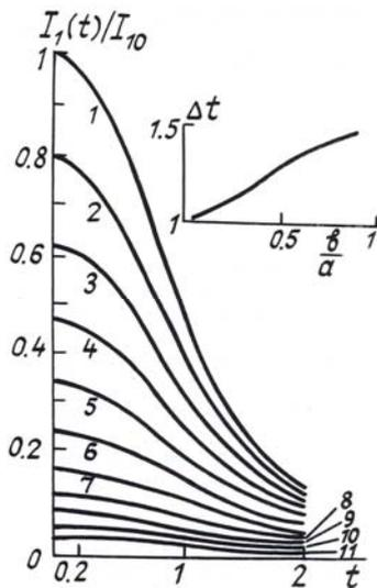
FIG. 1. The energy distribution in the ring bounding the central part of the irradiation spot for different values of  $b/a$ :  $b/a \neq 0$  (1), 0.1 (2), ... 1 (11). The width of the ring  $\Delta t$  as a function of the parameter  $b/a$  is shown in the inset.
