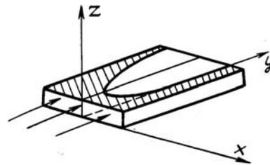
FIG. 1. Beam, path for the LiNbO<sub>3</sub> crystal. The axes correspond to the notation:  $x - 1$ ,  $y - 2$ ,  $z - 3$ .
