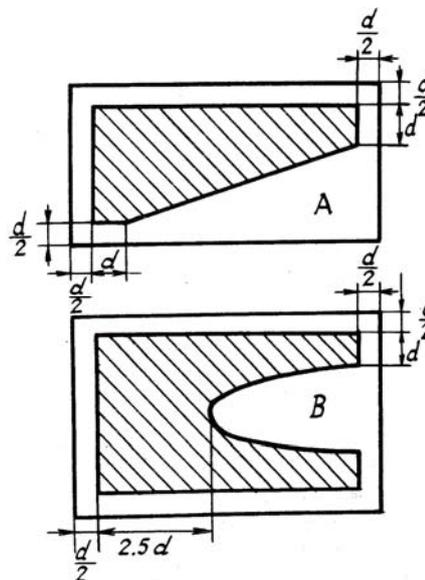
FIG. 3. Electrode shapes for  $\text{LiNbO}_3$  samples,  $d$  is the crystal thickness
