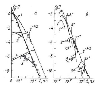
FIG. 4. Pulse shapes obtained by numerical calculations (a) and by SADA (b) for different detector angular displacements from the beam axis:  $1 - \alpha = 0.5^{\circ}$ ;  $2 - \alpha = 2^{\circ}$ ;  $3 - \alpha = 10^{\circ}$ .
