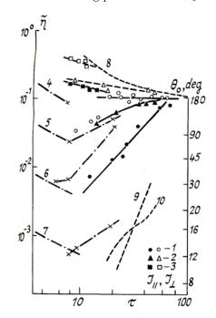
FIG. 2. The pulse width expressed in terms of the parameter  $\tilde{\eta}$  as a function of the optical thickness of the layer. Experiment – curves 1–3. Calculation:  $\alpha = 10^{\circ}$ ,  $4 - \omega = 80^{\circ}$ ,  $5 - \omega = 10^{\circ}$ .  $6 - \omega = 1^{\circ}$ ,  $7 - \alpha = 2^{\circ}$ ,  $\omega = 2^{\circ}$ .
