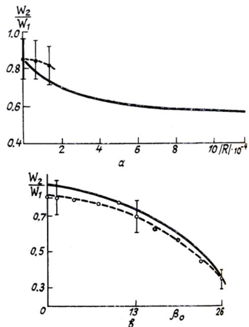
FIG. 3. Calculated (solid curve) and experimental (dashed curve) values of the correction parameter  $W_2/W_1$  as a function of the parameters  $R$  (a) and  $\beta_0$  (b).
