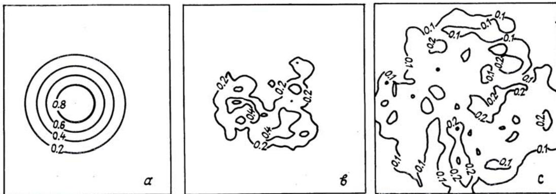
FIG. 4. Computed contour lines of normalized beam intensity for the probe beam at  $z = 0$  (a) and  $z = L_1$  (b) and the conjugate beam in the plane  $z = 0$  for  $\tilde{g} = 20$  (a) and 80 (c).
