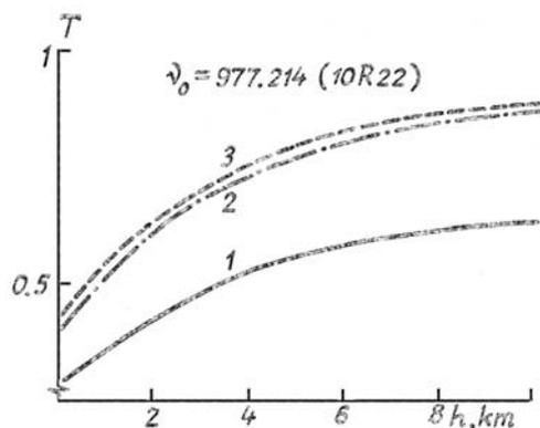
FIG. 3. Transmission of the atmosphere along a vertical path as a function of the lower endpoint height.
