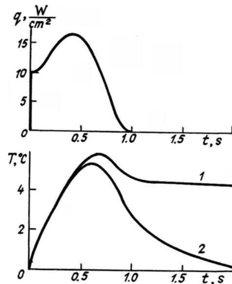
FIG. 1. Time dependence of the surface temperature of heat-insulated, (1) and cooled (2) sections of the target when it is exposed to pulse of laser radiation.
