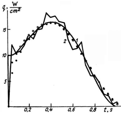
FIG. 2. Retrieving model dependence (20) of  $q(t)$  from the surface temperature of cooled target: 1) exact solution; 2) use of interpolating splines. Dots indicate the smoothed solution on the basis of Eq. (10) and circles – of Eq. (17).
