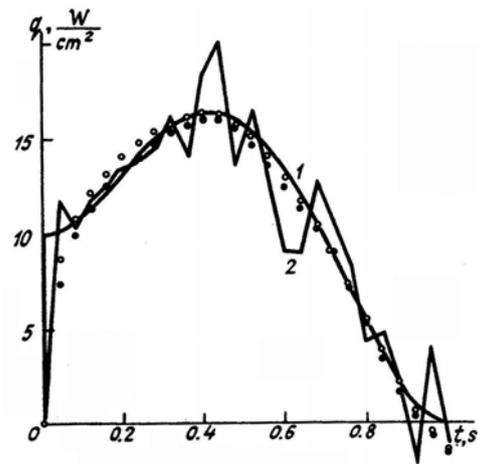
FIG. 3. Retrieving model dependence (20) of  $q(t)$  from the surface temperature of heat-insulated target: 1) exact solution; 2) use of interpolating splines. Dots indicate the smoother solution based on Eq. (14) and circles – on Eq. (19).
