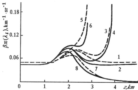
FIG. 1. Examples of the instability of the solutions caused by the error  $\Delta\beta(\lambda_i, 0)$  at the reference point  $z_p=0$ . Curves 1 and 2 represent model profiles of  $\beta(\lambda_i, z)$  and 3 and 4 represent the reconstructed profiles.  $\Delta\beta(\lambda_i, 0) = 0.5$  (3 and 4), 2 (5 and 6), and  $-2\%$  (7 and 8).
