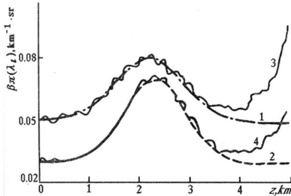
FIG. 3. Numerical simulation of processing of data of bifrequency sounding with the help of the algorithm at  $\tau \approx 5$ : 1), 2) model profiles  $\beta(\lambda_i, z)$  and 3), 4) reconstructed profiles.
