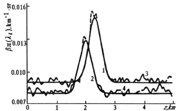
FIG. 2. Numerical simulation of processing of bifrequency sounding data with the help of the proposed algorithm at  $\tau \approx 1$ ; 1), 2) model profiles of  $\beta(\lambda_i, z)$ , and 3), 4) the reconstructed profiles.
