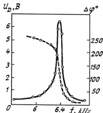
FIG. 3. The frequency (solid line) and phase (dashed line) responses of the OAD measured at a pressure of 0.5 Torr for pure  $\text{CH}_3\text{OH}$  for the lasing line of the  $\text{CO}_2$  laser 9P(16).  $U_D$  is the voltage at the detector output and  $\Delta\zeta$  is the phase of the opto-acoustic signal.
