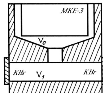
FIG. 1. The design of the detector with the Helmholtz cavity;  $V_0$  is the volume of the cavity and  $V_1$  is the volume of the channel for the laser transmitted radiation.
