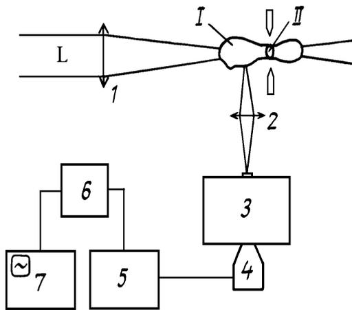
FIG. 2. Block diagram of the experimental setup for studying the spectrum dynamics of plasma: L refers to the radiation of a GOS-1001 laser, I – to t plasma of discharge, II – to t plasma seed initiating the breakdown spark. 1) lens with  $f = 25$  cm, 2) INDUSTAR-51 objective lens; 3) CDMC monochromator; 4) LI-602 dissector; 5) control unit; 6) GI-1 pulse oscillator; 7) S9-8 storage oscillograph.
