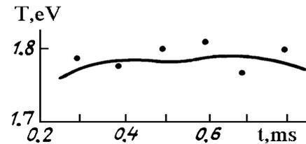
FIG. 3. Time dependence of the plasma temperature at a distance of  $10 \mu\text{m}$  from the focal point.
