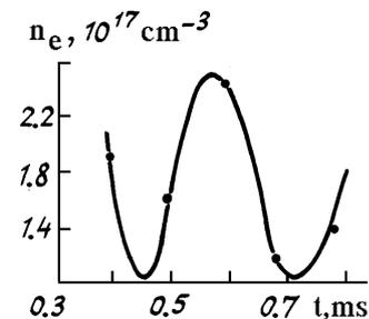
FIG. 4. Time dependence of the electron number density of discharge at a point located at a distance of  $3 \mu\text{m}$  from the focal point.
