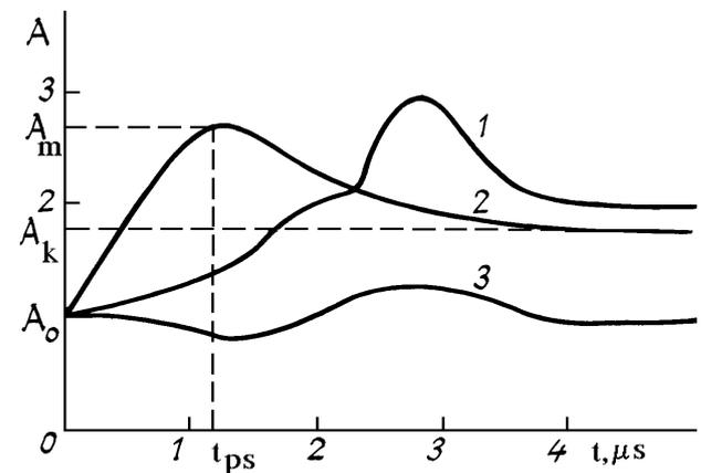
FIG. 1. Time dependence of the amplitude of the signal at  $\lambda = 0.49 \mu\text{m}$  caused by scattering of a probing beam with different energy densities: 1) 4 J/cm<sup>2</sup>, 2) 17 J/cm<sup>2</sup>, and 3) 2 J/cm<sup>2</sup>.
