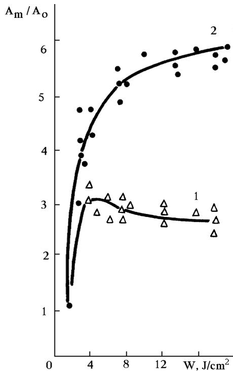
FIG. 2. The dependence of the maximum amplitude of the scattered signal at  $\lambda = 0.49 \mu\text{m}$  on the energy density in the beam of the  $\text{CO}_2$ -laser radiation: polydisperse aerosol approximated by the gamma distribution with the parameters  $a_m = 4 \mu\text{m}$  and  $\mu = 1$  (1) and  $a_m = 10 \mu\text{m}$  and  $\mu = 1.21$  (2).
