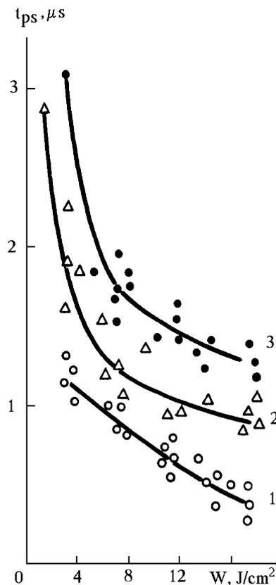
FIG. 3. The dependence of the time for the amplitude of the scattered signal to reach its peak value on the energy density in the pulse of the  $\text{CO}_2$  laser: monodisperse aerosol with  $\bar{a} = 2.7 \mu\text{m}$  (1), polydisperse aerosol approximated by the gamma distribution with the parameters  $a_m = 4 \mu\text{m}$  and  $\mu = 1$  (2), and  $a_m = 10 \mu\text{m}$  and  $\mu = 1.21$  (3).
