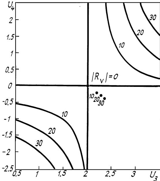
FIG. 1. Coordinates of the minimum of functional of focusing  $\hat{F}_3$  and curves of zero functional of astigmatism  $\hat{F}_4$  in the plane of modal control  $(U_3, U_4)$  for different values of the nonlinearity parameter  $R_v$ . Path length  $z = 0.5\kappa a_0^2$ .
