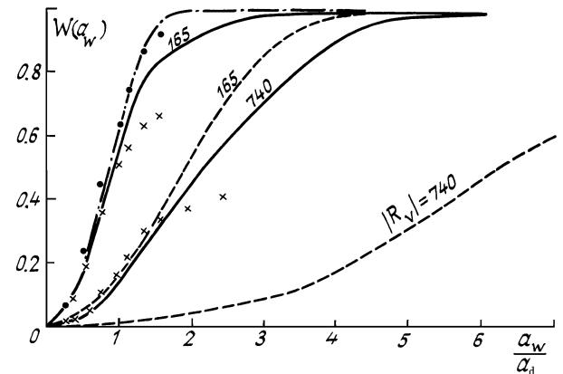
FIG. 5. Normalized power  $W(a_W)$  vs. receiving aperture radius  $a_W$ .  $a_d$  is the diffraction radius of a Gaussian beam. Data are obtained from the digitized image: dash-dot line shows the linear case  $R_v = 0$ , dashed line shows the "off" mode of control; solid line shows the "on" mode of control. The PM data: dots indicate the linear case and crosses show the corresponding parameter after the control.
