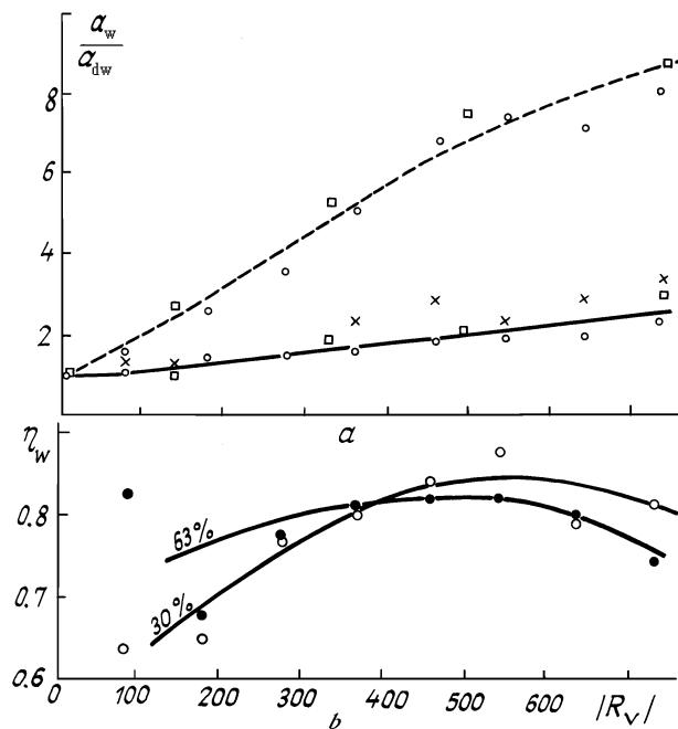
FIG. 6. Energetic radius of the beam  $a_W$ . a) Energetic radius  $a_W$  at 63% level of the total power vs  $R_v$ . Empty circles and crosses: flow speed  $v = 2$  mm/s; squares:  $v = 1.1$  mm/s; dashed lines: without control; solid lines: after control. Clear circles and squares: digitized image; crosses: PM data. b) Energetic efficiency of control  $\eta_w$  vs the parameter of nonlinearity  $R_v$  at 63% and 30% levels of the total power and for the flow speed  $v = 2$  mm/s.
