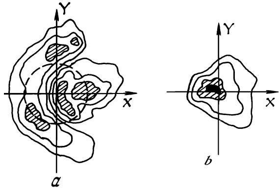
FIG. 4. Intensity isophotes in the beam cross-section (far zone of diffraction) for  $|R_v| = 640$ . a) in the "off" mode of control; b) in the "on" mode of control. The origin of the coordinate system coincides with the beam energy center  $(x_c, y_c)$ . Dashed curve shows the receiving aperture.
