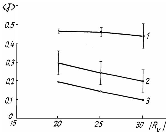
FIG. 4. The resultant values of the criterion of focusing  $J$  averaged over 30 iterative steps vs the nonlinearity of the medium in the case of stationary refraction at  $z_0 = 0.5 z_d$ : 1) two-mirror system, 2) phase conjugation and 3) without control.
