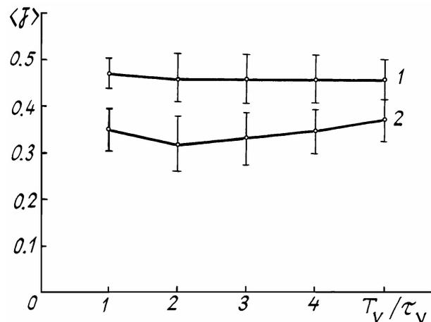
FIG. 5. Adaptive control in the presence of pulsations of the wind velocity. The quality of correction of thermal blooming vs the period of wind velocity pulsations  $T_v$ ,  $z_0 = 0.5 z_d$  and  $\langle R \rangle = -20$ . The interval of time averaging is about  $40 \tau_v$ : 1) adaptive two-mirror system and 2) algorithm of cross-aperture sensing.
