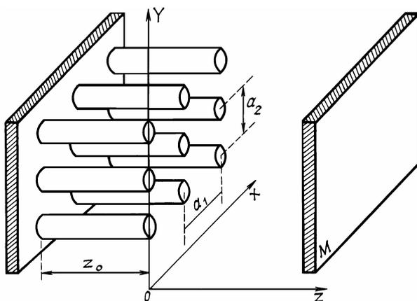
FIG. 1. Diffraction-coupled laser array.  $M$  is the coupling mirror.
