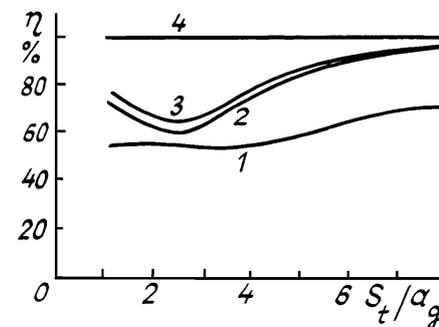
FIG. 4. The normalized criterion of correction quality  $\eta$  as a function of the radius of receiving aperture  $S_t$  for different number of the controllable modes. 1) without correction, 2) second-order modes, and 3, 4) third- and fourth-order modes, respectively. Path length  $z_0 = 0.2$  and the nonlinearity parameter  $R = -100$ .
