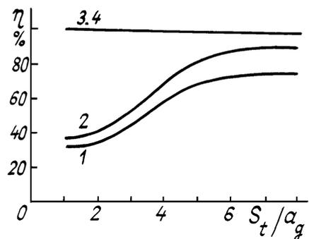
FIG. 2. The normalized criterion of correction quality  $\eta$  as a function of the radius of the receiving aperture  $S_t$  for different number of the modes. 1) without correction, 2) second-order modes, and 3, 4) third- and fourth-order modes, respectively. Path length  $z_0 = 0.5$  and the nonlinearity parameter  $R = -40$ .
