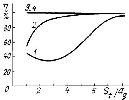
FIG. 1. The normalized criterion of correction quality  $\eta$  as a function of the radius  $S_t$  of the receiving aperture for different number of the controllable modes. 1) without correction, 2) second-order modes, and 3, 4) third- and fourth-order modes, respectively. Path length  $z_0 = 0.5$  and the nonlinearity parameter  $R = -20$ .
