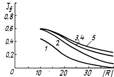
FIG. 3. The criterion of focusing  $J_f$  within the circle of radius  $S_t = 2a_d$  as a function of the nonlinearity parameter  $R$ . 1) without correction, 2) second-order mode, 3, 4) third- and fourth-order modes, respectively, and 5) ideal corrector. Path length  $z_0 = 0.5$ .
