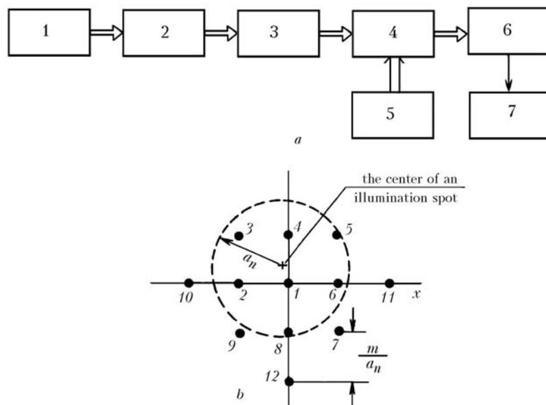
FIG. 1. Block diagram of the experimental setup (a): 1) laser, 2) diaphragm, 3) transfer power meter, 4) directing mirror, 5) control unit for the mirror, 4, 6) target, and 7) computer. The scheme of RD positions (b): 1–12 are the fixed points for recording the optical signal.
