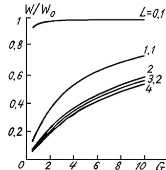
FIG. 3. The family of the dependencies of the displacement  $W/W_0(G)$  of the actuator transferred through the layered substrate of the active mirror on the relative stiffness of the actuator  $G$  for different values of  $L$ .
