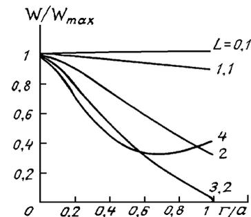
FIG. 2. The typical response functions of the active mirror against the parameter  $L$ .
