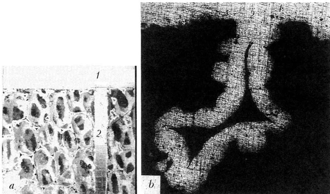
FIG. 4. Photomicrograph of the experimentally realized structure of the composite copper substrate of the active mirror: a) compact layer (substrate of the mirror) (1) and model of the actuator case (2) and b) joint of the compact substrate of the specular surface and the elastic permeable sublayer fabricated from the HPM.
