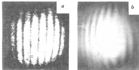
FIG. 4. Shear interferograms with the spatial filtration in the image plane of the mat screen: a) on the optical axis and b) off the optical axis.
