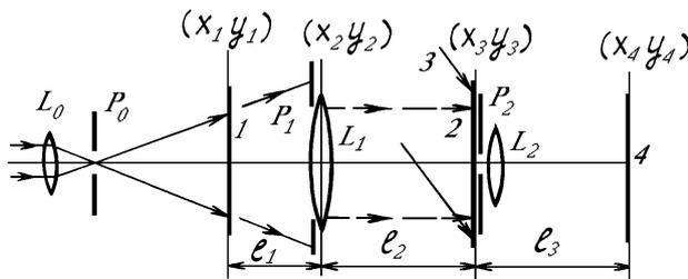
FIG. 1. The optical scheme used for recording and reconstructing a doubly exposed hologram: 1) mat screen; 2) photographic plate-hologram; 3) reference beam; 4) recording plane of the interferogram;  $L_0$ ,  $L_1$ , and  $L_2$  are lenses;  $p_1$  and  $p_2$  are aperture diaphragms; and,  $p_0$  is a spatial filter.
