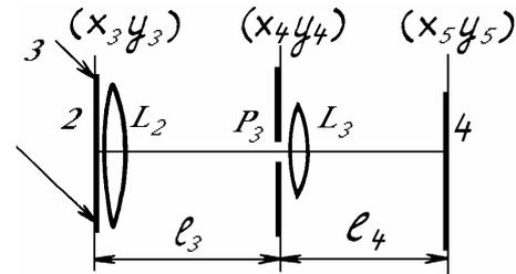
FIG. 2. The optical scheme used for recording of the interference pattern localized in the hologram plane when spatial filtering is performed in the image plane of the mat screen.
