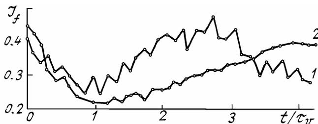
FIG. 3. Dynamic control of the beam phase based on the simplex method for two values of the simplex edge length:  $L = 0.6$  (curve 1) and  $0.3$  (curve 2). Parameters of propagation:  $z_0 = 0.5$  and  $R = -20$ .
