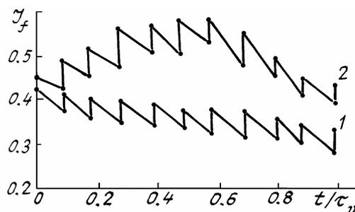
FIG. 4. Beam phase control for "frozen" instantaneous states of the medium ( $\tau_c = 0.01\tau_v$ ). 1)  $L = 0.1$  and 2)  $L = 0.2$ . Parameters of propagation:  $z_0 = 0.5$  and  $R = -20$ .
