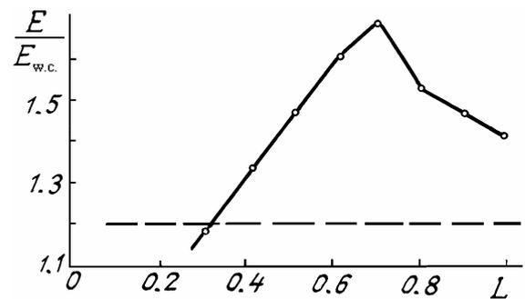
FIG. 2. The total relative light energy  $E/E_{w.c.}$  falling within the receiving aperture during the control time  $T = 3\tau_v$  as a function of the simplex edge length  $L$  (dashed line is for the gradient method with an optimal step). Parameters of propagation:  $z_0 = 0.5$  and  $R = -20$ .  $E_{w.c.}$  is the energy in the system without control.
