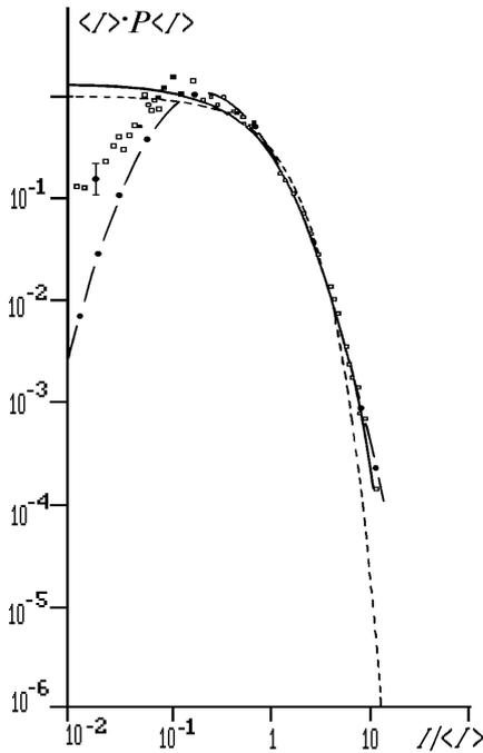
FIG. 1. A comparison of the histogram of the normalized intensity with the lognormal distribution (curve 1), exponential distribution (curve 2), and K-distribution (curve 3) for  $\beta_0 = 11.5$  and  $\beta = 1.18$  in the range  $0.01 \leq I / \langle I \rangle \leq 15$  for a plane wave.
