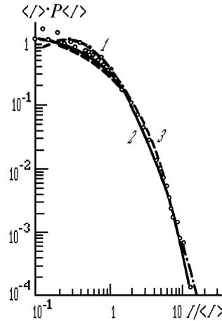
FIG. 2. A comparison of the histogram of the normalized intensity with the lognormal distribution (curve 1), K-distribution (curve 2), and Weibull distribution (curve 3) for  $\beta_0 = 11.5$  and  $\beta = 1.18$  in the range  $0.1 \leq I / \langle I \rangle \leq 15$  for a plane wave.
