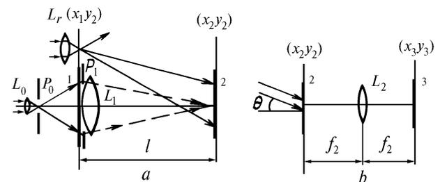
FIG. 1. The scheme for recording (a) and reconstructing (b) a three-exposure lens Fourier hologram: 1) mat screen; 2) photographic plate-hologram; 3) recording plane of the interference pattern;  $L_0$ ,  $L_r$ ,  $L_1$ , and  $L_2$  are lenses;  $p_0$  is a spatial filter; and  $p_1$  is aperture diaphragm.
