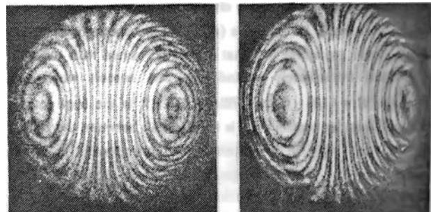
FIG. 2. Shear interferograms recorded during spatial filtering in the plane of the hologram: a) on the optical axis and b) off the optical axis.
