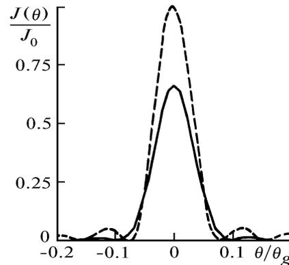
FIG. 5. Directional pattern of radiation for  $N = 10$ ,  $a/\sigma = 4$ , and  $G_0 = 0.7$ : cophased collective generation (solid curve) and cophased sources of equal amplitude (dashed curve).
