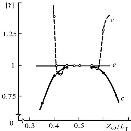
FIG. 4. Modulus of eigenvalues of cophased (*c*) and antiphased (*a*) collective modes vs the distance to the coupling mirror. Linear case ( $G_0 = 0$ ):  $a/\sigma = 4$  (solid curve) and  $a/\sigma = 8$  (dashed curve). Nonlinear case:  $G_0 = 0.7$  and  $a/\sigma = 4$  (filled circles);  $G_0 = 2$  and  $a/\sigma = 8$  (empty circles).
