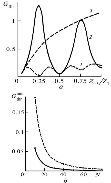
FIG. 2. Threshold gains  $G_{\text{thr}}$  for cophased and antiphased collective modes: a)  $G_{\text{thr}}$  vs the distance  $z_{\text{co}}$  to the coupling mirror for  $a/\sigma = 4$  and  $N = 10$  for antiphased (1), cophased (2), and independent (3) generations of the laser array and b)  $G_{\text{thr}}$  vs the number of lasers  $N$  in the array for  $z_{\text{co}} = z_T/2$ ,  $a/\sigma = 4$  (solid curve), and  $a/\sigma = 8$  (dashed curve).
