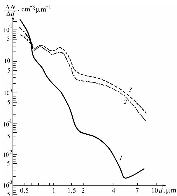
FIG. 8. Aerosol particle size distribution in the Amursk plume at a distance of 1) 2 km, 2) 20 km, and 3) 22 km from the edges of stacks.
