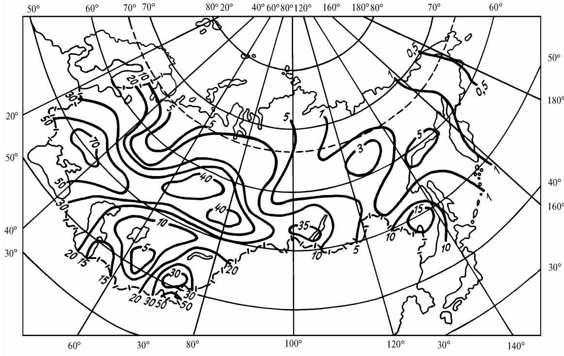
FIG. 1. Distribution of aerosol number density ( $\bar{N} = \frac{1}{H} \int_0^H N(h)_i dh$ ) over the territory of the former USSR.
