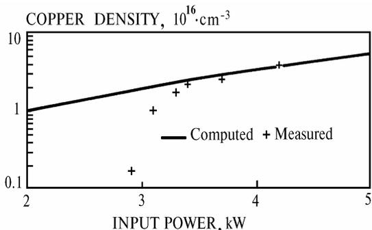
FIG. 2. Density produced by copper vapor generator.
