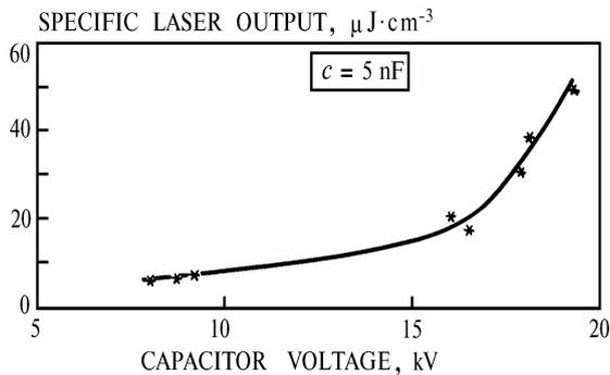
FIG. 4. Specific output rises with capacitor voltage.
