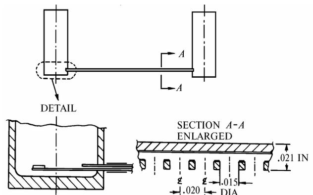
FIG. 1. Schematic of copper vapor generator.
