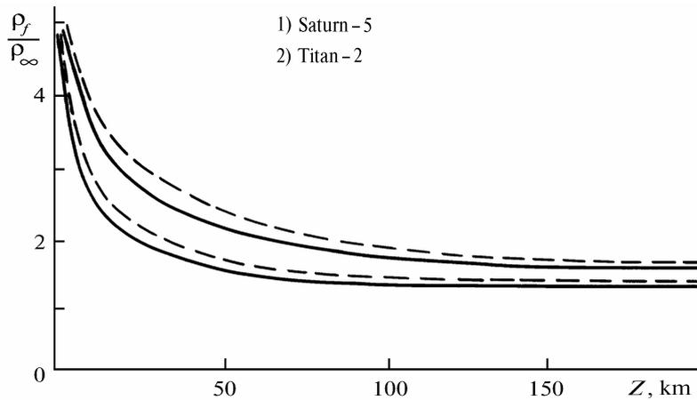
FIG. 4. Densities of particle condensation along the rocket flame axis at an altitude of 150 km at  $v_{roc} = 3$  (solid line) and 5 km/s (dashed line).
