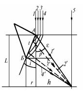
FIG. 1. The scheme of diffraction of a parallel light beam by a thick screen.
