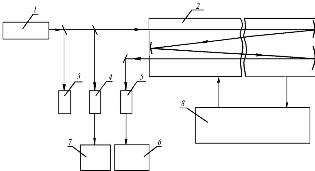
FIG. 1. Block diagram of the laser spectrophotometer: 1) laser, 2) multipass gas absorption cell, 3) wavelength meter, 4 and 5) photodetectors, 6 and 7) digital voltmeters, and 8) system for preparing and control of gas mixtures.
