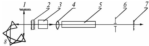
FIG. 4. Optical arrangement of a neodymium glass laser: 1 and 7) resonator mirrors, 2) Fabry-Perot etalon, 3) passive Q-switch, 4) lens, 5) active element, 6) diaphragm, and 8) block of dispersion prisms.
