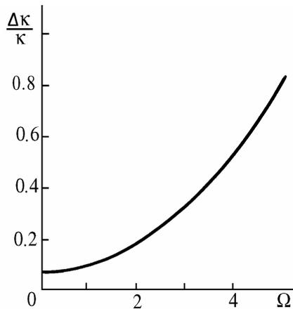
FIG. 2. Dependence of relative error in measurements of the absorption coefficient on the frequency detuning from an absorption line center.
