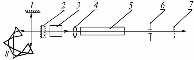
FIG. 4. Optical arrangement of a neodymium glass laser: 1 and 7) resonator mirrors, 2) Fabry-Perot etalon, 3) passive Q-switch, 4) lens, 5) active element, 6) diaphragm, and 8) block of dispersion prisms.
