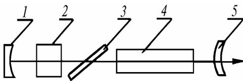
FIG. 3. Optical arrangement of an Nd:YAG laser: 1) concave mirror, 2) passive Q-switch, 3) polarizer, 4) active element, and 5) convex mirror.
