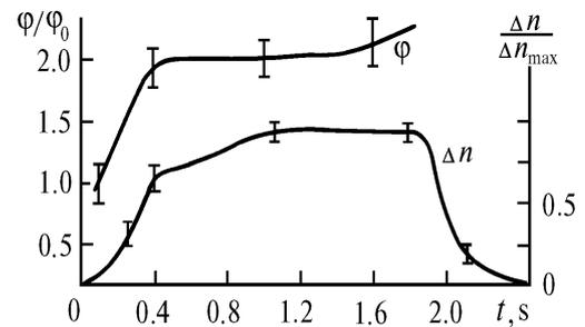
FIG. 2. A comparison between the angular size of the HPR beam at the far end of the path and variation in  $\Delta n$  inside the active channel.
