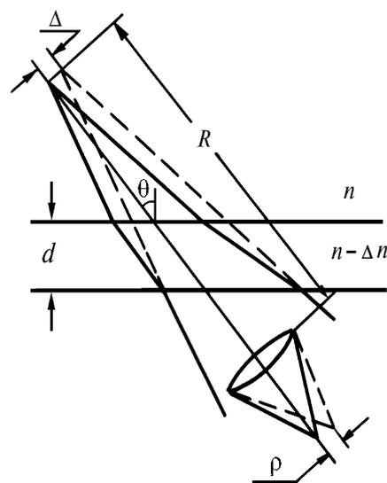
FIG. 1. Diagram for determining the variation in the refractive index.
