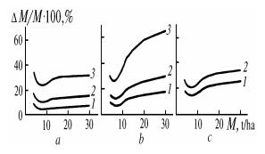
FIG. 5. Effect of measurement errors of the MSS apparatus (in the second and fourth channels) on the accuracy of reconstruction of vegetation biomass: a) with measurement errors  $\delta L_1$  in the second channel being equal to 5, 10, and 20%, respectively (curves 1–3); b) with  $\delta L_2$  for the first channel being equal to 3, 5, and 10% (curves 1–3); and, c) with  $\delta L_1 = 5\%$  and  $\delta L_2 = 3\%$  (1) and  $\delta L_1 = 10\%$  and  $\delta L_2 = 3\%$  (2).
