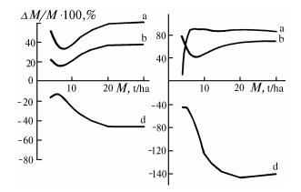
FIG. 3. The effect of inexact knowledge of the atmospheric properties (types a, b, and d) at the instant of imaging on the reconstruction of the vegetation biomass with the help of the approximation coefficients corresponding to the atmospheric conditions of the type c for the second and fourth (to the left) and first and third (to the right) channels of the MSS.
