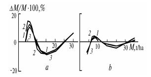
FIG. 2. Theoretical systematic errors of the proposed method of reconstructing the amount of vegetation biomass for the AVHRR apparatus and the second and fourth and first and third channels of the MSS (curves 1, 2, and 3) in the case of approximation of the parameter M in terms of  $G^*$  by polynomials of the fourth (a) and third (b) degrees.
