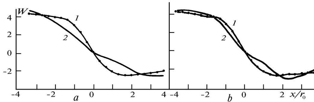
FIG. 4. Bending of the mirror reconstructing the phase surface (section by the ZOx plane). Curve 1 represents the profile of the phase surface and curve 2 represents the mirror profile. (a) is for servodrive configuration b from Fig. 1 and (b) for the configuration c from Fig. 1. Parameters used:  $z_{NL} = 0.1$ ,  $z_L = 0.4$ , and  $R_v = -90$ .
