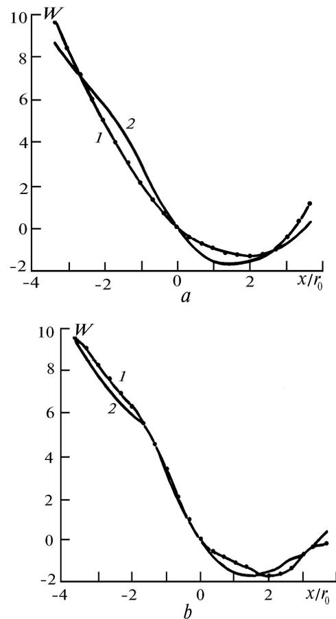
FIG. 3. Bending of the mirror reconstructing the correcting phase surface (section by the ZOZ plane). Curve 1 represents the profile of the phase surface, while curve 2 shows the profile of the mirror. (a) is for servodrive configuration b from Fig. 1 and (b) for the configuration c from Fig. 1. Parameters used:  $z_{NL} = 0.5$ ,  $z_L = 0$ , and  $R_v = -30$ .
