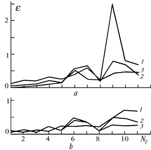
FIG. 2. Accuracy of Zernike polynomials reconstruction with mirrors *b* (*a*) and *c* (*b*) from Fig. 1:  $\epsilon$  is the rms error,  $N_z$  is the number of the Zernike polynomial to be reconstructed,  $r_f = 1/10 d_m$  (curve 1),  $r_f = 1/5 d_m$  (curve 2), and  $r_f = 1/2 d_m$  (curve 3).
