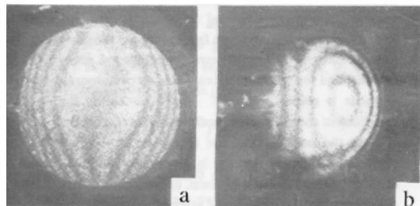
FIG. 3. Shear interferograms characterizing: a) phase distortions of the illuminating wavefront and b) phase distortions of the reference beam.
