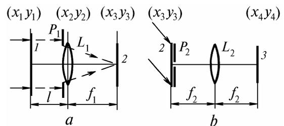
FIG. 1. The scheme used for recording (a) and reconstruction (b) of a double-exposure Fourier hologram of the mat screen: 1) mat screen, 2) photographic plate-hologram, 3) recording plane of the interferogram;  $L_1$  and  $L_2$  are lenses;  $P_1$  is the aperture diaphragm; and,  $P_2$  is the filtering diaphragm.
