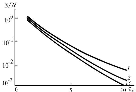
FIG. 3. The  $S/N$  ratio depending on the optical depth of layered inhomogeneous medium at  $\Lambda = 1$ : 1)  $\tau_y = \tau_z = 1$ , 2)  $\tau_y = \tau_z = 5$ , and 3)  $\tau_y = \tau_z = 10$ .
