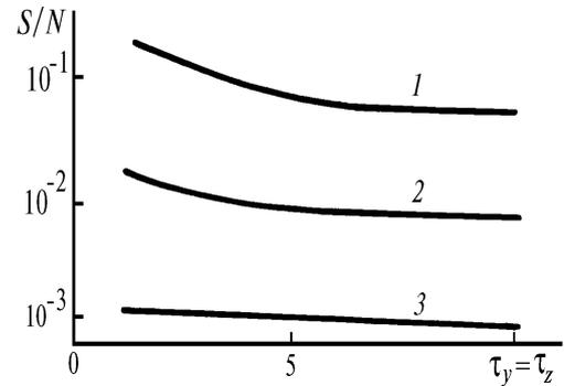
FIG. 1. Signal-to-noise ratio depending on the transverse optical dimensions of the medium at  $\Lambda = 0.8$  and  $\tau_x = 10$ : a = 1 (1), layered medium (2), and a = 12.09 (3).
