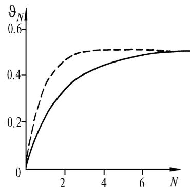
FIG. 2. A plot of the value of initial beam focusing vs a number of iterations for  $\alpha = -10$ ,  $l = 0.25$ , and  $\vartheta_0 = 0$ . Solid curve illustrates calculations using the method described; dashed curve the calculations using the Fourier transform technique.
