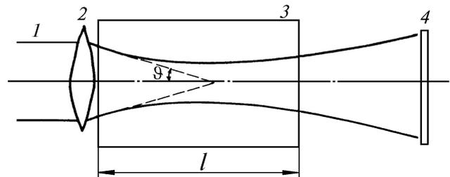
FIG. 1. Scheme of the problem under study: 1) laser beam; 2) controllable lens; 3) nonlinear medium; and 4) receiver in the far diffraction zone.
