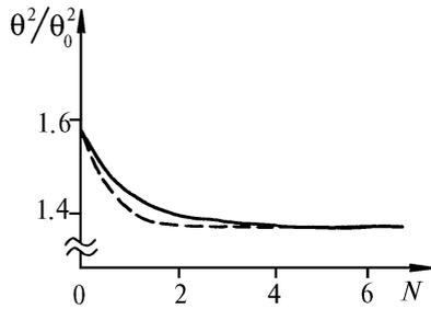
FIG. 3. A plot of the normalized quality criterion vs a number of iterations for  $\alpha = -10$ ,  $l = 0.25$ , and  $\vartheta_0 = 0$ . Solid curve is for calculations made using the method described; dashed curve is for calculations by Fourier transform ( $Q_0^2$  is the angular divergence in a linear medium).
