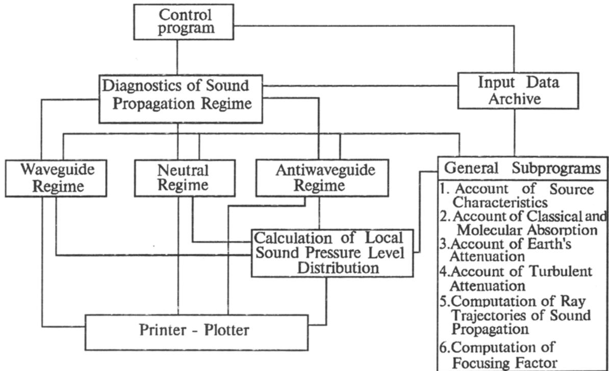
FIG. 1. Flowchart of the software package AOS (Acoustics of Open Space).
