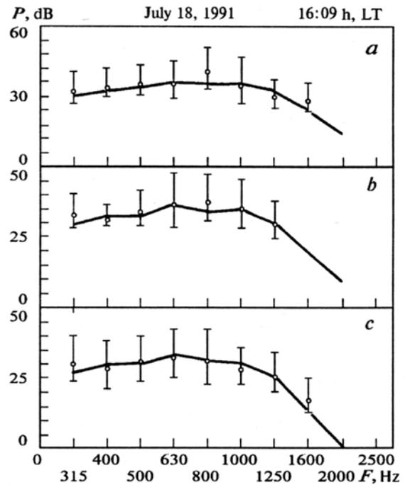
FIG. 4. Sound pressure level, in dB, in the case of antiwaveguide regime for various path lengths as a function of the frequency  $f$  of radiated signal,  $d = 3575$  m (a),  $4135$  m (b), and  $4800$  m (c). Solid lines are for the results of calculation, and circles are for the measured values. Vertical bars denote the confidence intervals.
