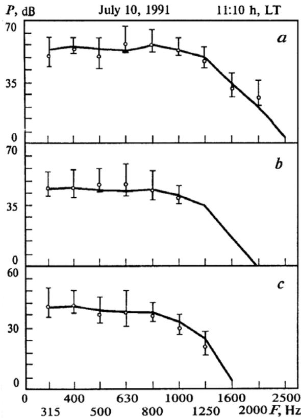
FIG. 3. Sound pressure level, in dB, in the case of waveguide regime for different path lengths as a function of the frequency  $f$  of radiated signal,  $d = 3000$  (a),  $4500$  (b), and  $6000$  m (c). Solid curves are for the calculated results; circles are for the measured values. Vertical bars denote the confidence intervals.
