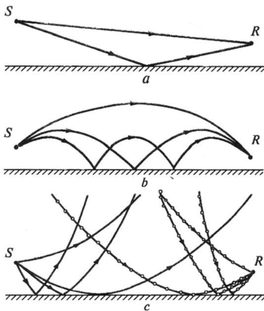
FIG. 2. Ray patterns for acoustic noise propagation in the atmosphere under various meteorological conditions: a) neutral regime; b) waveguide regime (only the top-bottom rays are shown); and, c) antiwaveguide regime. Here S is the noise source, R is the receiver (observation point), ----- — direct rays, -o-o-o- — the scattered rays.
