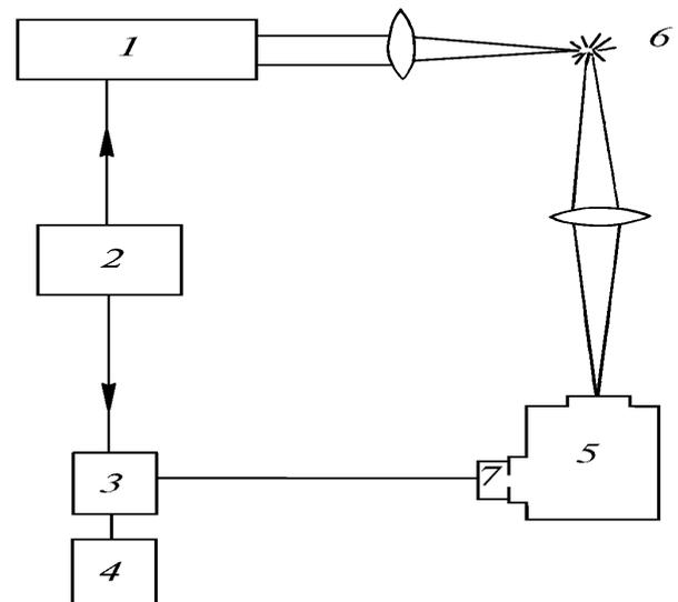
FIG. 1. Block diagram of a setup for analysis of laser spark. For spectrum recording we use the photodiode array operating during a fixed period after the breakdown initiation that allows the recording of the spark emission solely. Shown in the figure are a pulse laser (1), a control timer (2), a PD controller (3), an oscilloscope (4), a spectrograph (5), a laser spark (6), and a photodiode array (7).
