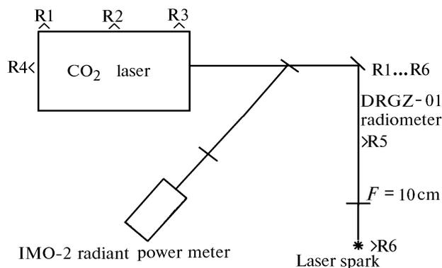
FIG. 1. Diagram showing the experimental configuration. Laser pulse energy is 6 J, radiant power density at the focus is  $10^9$  W/cm<sup>2</sup>.
